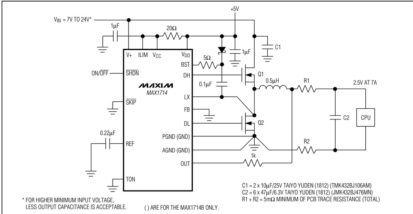
Figure 7. All-Ceramic-Capacitor Application
