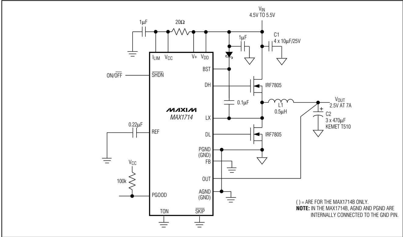
Figure 10. 5V Powered, 7A CPU Buck Regulator
