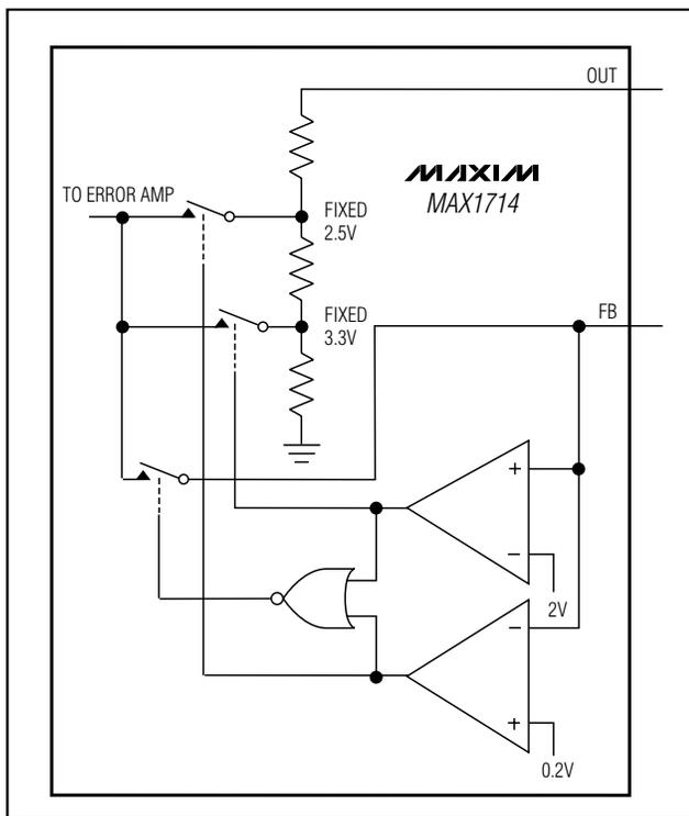
Figure 8. Feedback Mux
